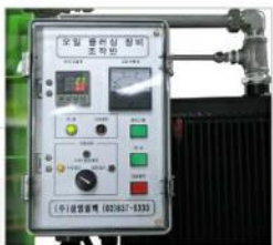
Control Panel Manually controls equipment operation and oil flushing
